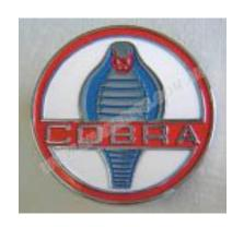
Cobra Bonnet & Boot Badges – The center of these badges were originally fitted 18 1/2" back from the forward edge of the boot lid and 11 1/2" forward of the front edge of the bonnet. Badges are centered on the boot and bonnet side to side.
